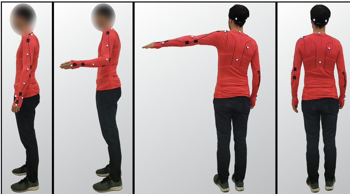
Figure S10: Side and rear view of the prototype garment, sensing fibre path, and OMC marker placement for some sample poses during the joint angle monitoring data collection.
