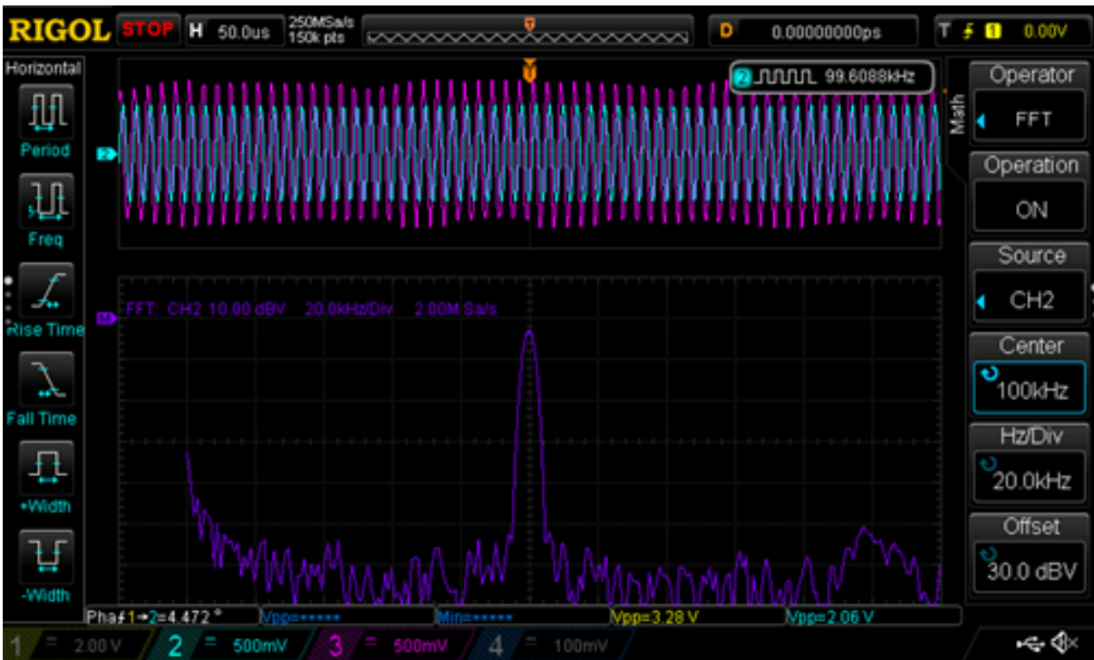
Figure S1: A frequency of 99.6 kHz was output by the SWG (the upper limit of the impedance analyzer design) and used to measure a signal-to-quantization noise ratio (SQNR) of approximately 58 dB and spurious-free dynamic range (SFDR) of 46 dB.
